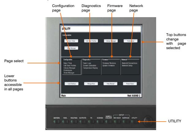
**The UTILITY front page** The screen is arranged with 4 main pages accessible by touching the big buttons in the centre of the screen. The top part of the screen changes according to page selected. The lower part presents the same set of buttons in all pages. These are the main operational UTILITY functions. Like the other screens, UTILITY always returns to the page last accessed. Touch the Return key at the top to navigate back to the top view and then on to the other pages.
